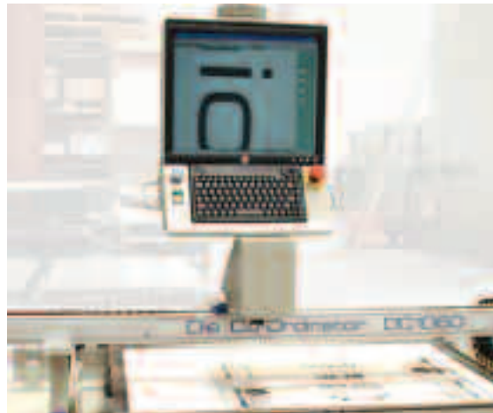
AutoScan scans images from the printed sheet to create keylines. Overcomes board stretch
