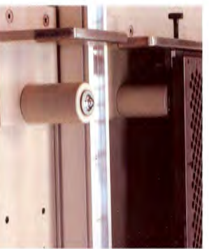
Adjustable Back Guides let you lock up any size of honeycomb off press.
