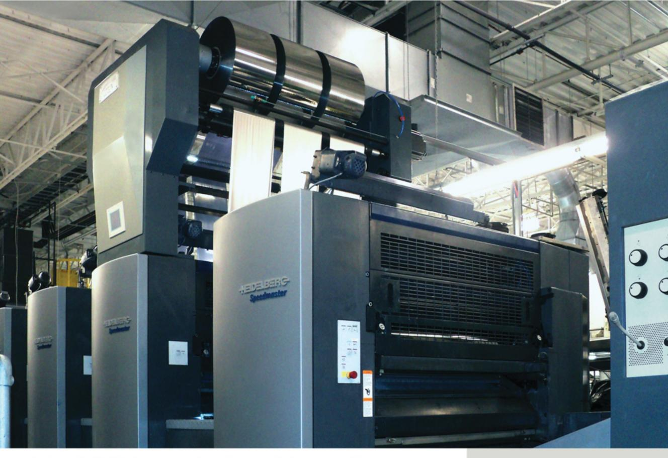
Indexing Cold Foil Technology is designed to work with almost any existing printing press. This Foildex™ is shown atop a Heidelberg press.
